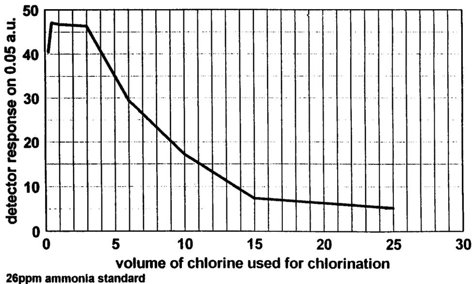
FIG. 2 Standard Preparation By the Chlorination of Ammonia
